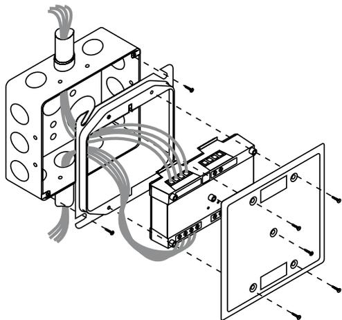
**SIGA-MCC1 and SIGA-MCC2:** mount the UIO motherboard inside a suitable EDWARDS enclosure with screws and washers provided. Plug the SIGA-MCC1 or SIGA-MCC2 into any available position on the motherboard and secure the module to the motherboard with the captive screws. Wiring connections are made to the terminals on the motherboard (see wiring diagram). UIO motherboard terminals are suited for #12 to #18 AWG (2.5 mm<sup>2</sup> to 0.75 mm<sup>2</sup>) wire size.
